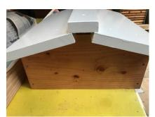
Measure the holes for the ridge. The ridge will need a very long screw (75 - 100mm) at each end. Use the drill bit to make the hole and mark where the screw will meet the gable. Remove the ridge to provide access to drill into the gable.
