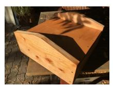
Square up the gables and side, clamp and screw. The ply cover needs to be well attached to the sides, so use screws to secure this part. This cover sits on the quilt box so takes some pressure. Once the roof is added it is difficult to repair the cover without dismantling the top.
